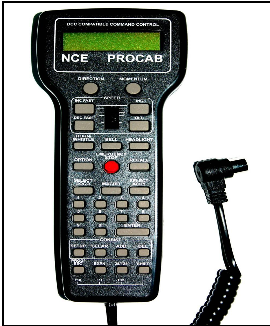
ProCab throttle with coiled cable and Right Angle DIN connector.
