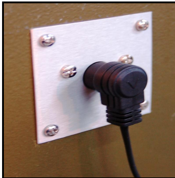
Right angle DIN connector correctly plugged into a fascia plate.
