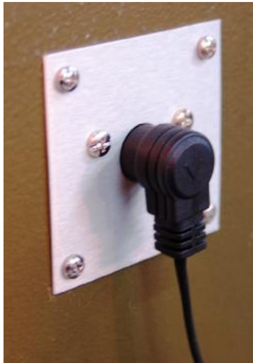
Right angle DIN connector correctly plugged into a fascia plate.
